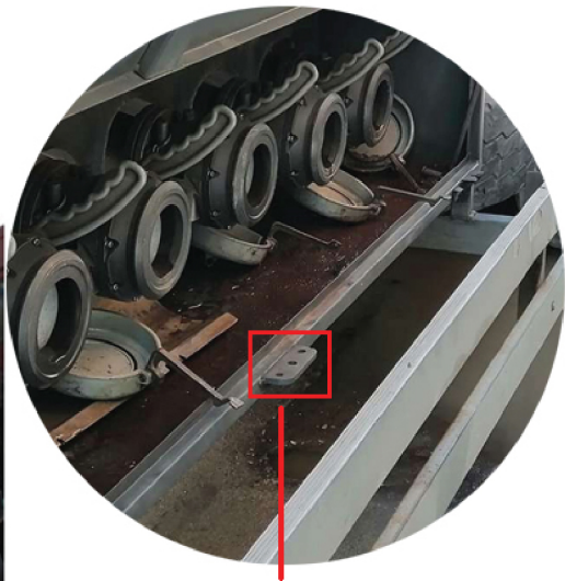
Lock cable go through these holes to lock the box
